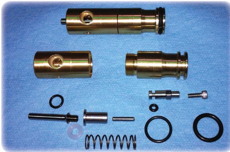
From top left down, is the valve body, breech seal, valve stem, pop-it seal, spring guide, stabilizer piston, valve spring, going back to the top right and coming down is the valve face, force reduction piston with seal, the seal between the two halves and the front seal.
